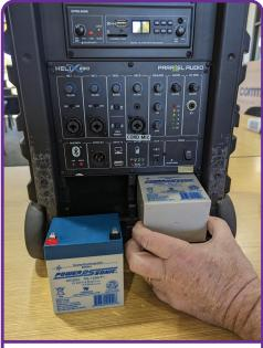
**6.** Place new batteries in compartment in same orientation that they were removed
