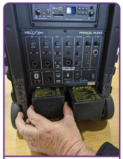
4. Remove existing batteries from the battery compartment
