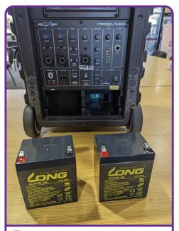
**5.** *Please Note:* Orientation of the battery terminals when removing exisiting batteries
